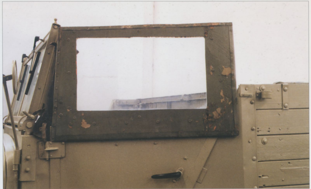
Door windows are made of transparent plastic and the frame is detachable. Lower picture shows the attachment of the front part of the canvas top. The canvas top itself is fixed to the wooden framing by means of straps. Clamps and plugs fasten the frame to the windshield.
