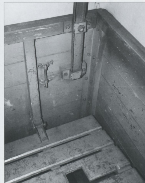
Compare the seat locking clamps shown here with the seat folded down with those on the page 44 (with the seat folded up).
