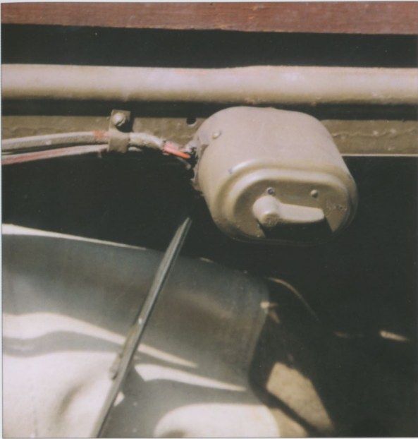
Original windshield wiper motors pictured above and below, were painted glossy black enamel. During actual vehicle service they were painted the body color.
