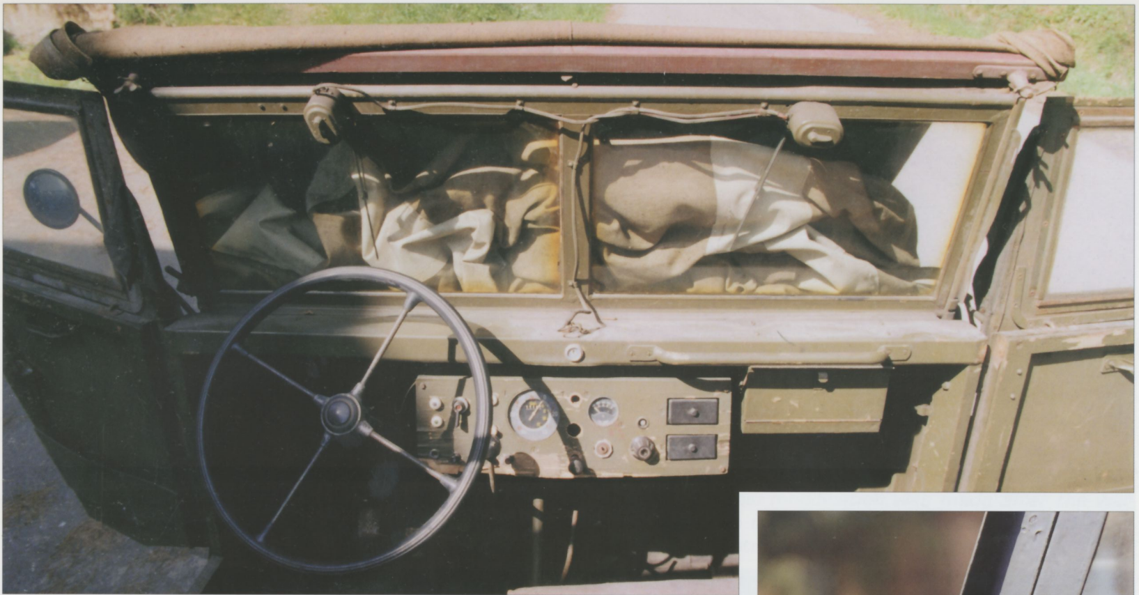
The dashboard shown on the top picture is not complete, probably due to a lack of original parts. Pictures on the bottom show door hinges and folding windscreen-locking mechanism.
