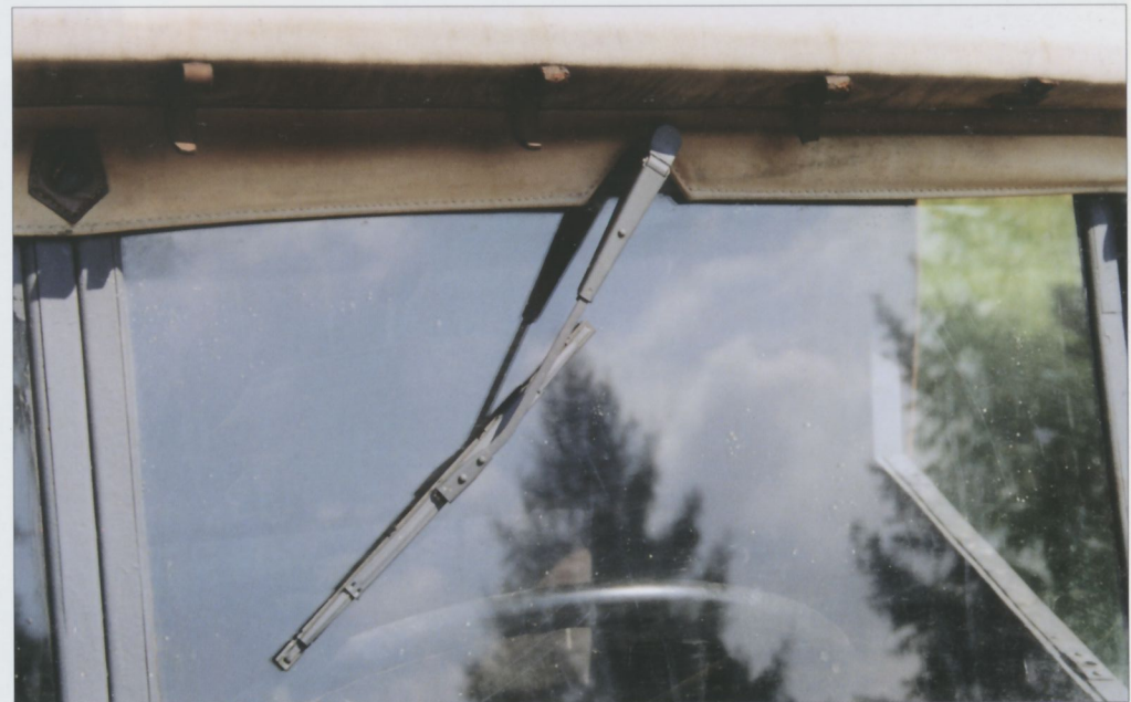
Door windows are made of transparent plastic and the frame is detachable. Lower picture shows the attachment of the front part of the canvas top. The canvas top itself is fixed to the wooden framing by means of straps. Clamps and plugs fasten the frame to the windshield.
