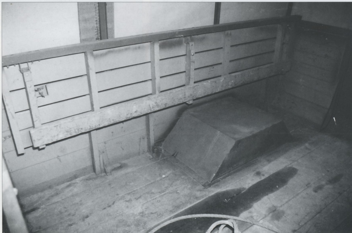
Compare the seat locking clamps shown here with the seat folded down with those on the page 44 (with the seat folded up).
