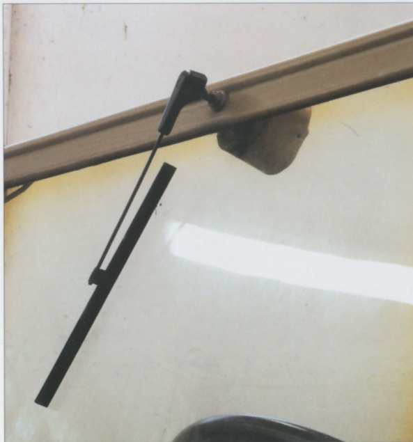
Original windshield wiper motors pictured above and below, were painted glossy black enamel. During actual vehicle service they were painted the body color.
